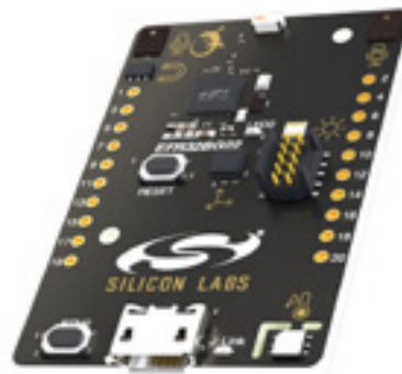
Fig. 6. The EFR32BG22 module is used in the Silicon Labs Bluetooth direction-finding solution. (Image: Press image: Silicon Labs)
